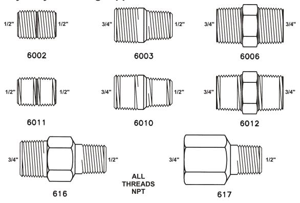
Sealco nipples are constructed of steel and plated with zinc and chromate for corrosion resistance
