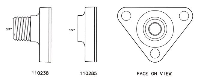
Flange Kits 0158H & 110285 are internally threaded. Flange Kits 110238 & 110285 include a washer.
