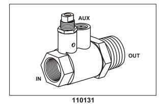
• Combination Valves act as a one-way check valve, pressure relief valve & manual drain
