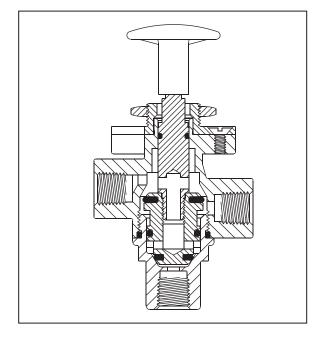
**INFORMATION:** • Commonly used as dash valve inside tractor, truck or dolly • Single hole mounting
